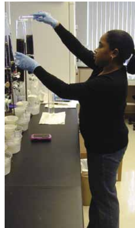
A USDA-ARS biological science technician measures nutrient release in greenhouse substrates amended with various forms and rates of biochar.
